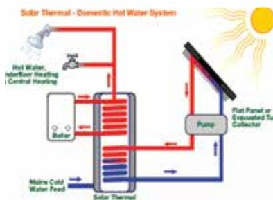
**Solar Thermal Water Heating System**
